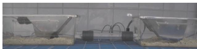
Figure 2 DoubleCage test unit: cage 1 and cage 2, perspex tunnel with two black sensors
